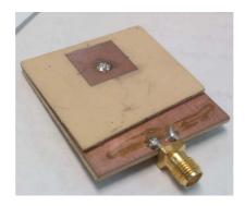
Figure 4. Fabricated single patch microstrip patch antenna.
