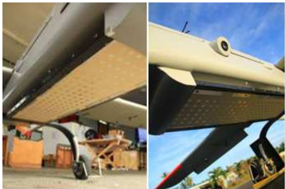
Figure 13. Mounting location of the antenna to the UAV.
