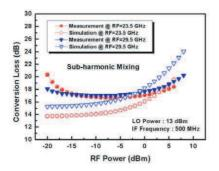
Figure 7. Measured and simulated conversion losses as functions of RF power.
