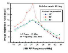
Figure 9. Measured IRR as a function of USB RF at different compensated phases.
