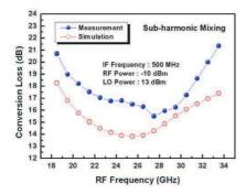
Figure 4. Measured and simulated conversion losses of the CMOS SHIRM as functions of RF at a fixed LO power of 13 dBmand an RF power of -10 dBm.
