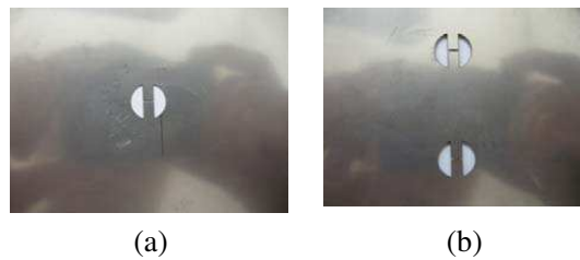
Figure 8. Photographs of apertures fabricated on a stainless steel plate: (a) Single aperture. (b) Dual apertures ( Y_d = 29\text{ mm} ).
