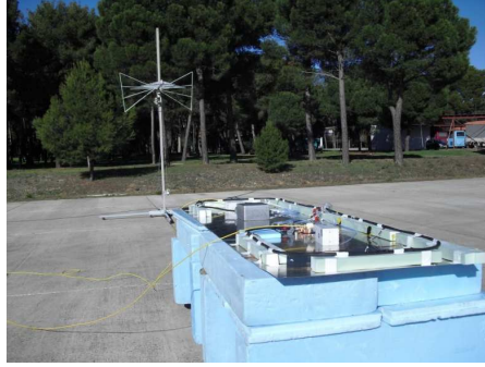
Figure 1. Experimental setup with the EMCO antenna at the INTA open-area test-site facility.
