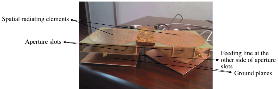
Figure 6. The spatial R-RLSA antennas with rice husk element.
