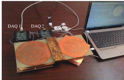
Figure 10. The fabricated integration of reconfigurable RLSA antennas into NI-DAQs.
