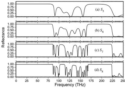
**Figure 4.** Normal incident reflection spectra for the different Fibonacci orders as a function of the frequency with (a)  $S_5$ , (b)  $S_6$ , (c)  $S_7$ , and (d)  $S_8$ .
