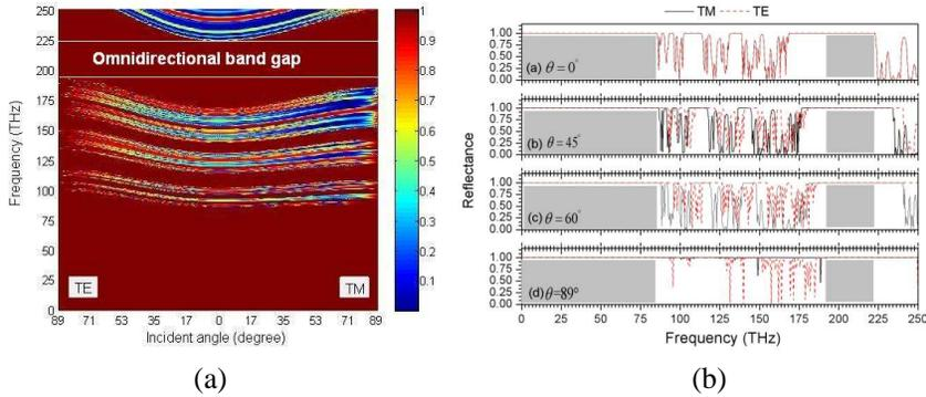
**Figure 3.** (a) Photonic band structure of 1D Fibonacci quasi-periodic SDPCS in terms of angular frequency and incidence angle. The areas between two white lines are the total OBG, and (b) reflectance spectra of 1D Fibonacci quasi-periodic SDPCS at various incident angles is calculated by TMM. The black solid (red dash dot) curves are for TM (TE) polarization, and the gray areas correspond to the PBGs.
