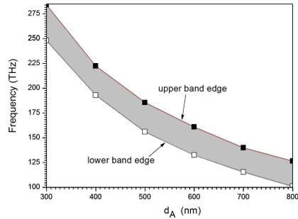
**Figure 9.** The frequency range of OBGs for Fibonacci quasi-periodic 1D SDPCs as a function of thickness of dielectric layer. The gray area is OBG.
