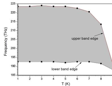
**Figure 11.** The frequency range of OBGs for Fibonacci quasi-periodic 1D SDPCs as a function of the ambient temperature. The gray area is OBG.
