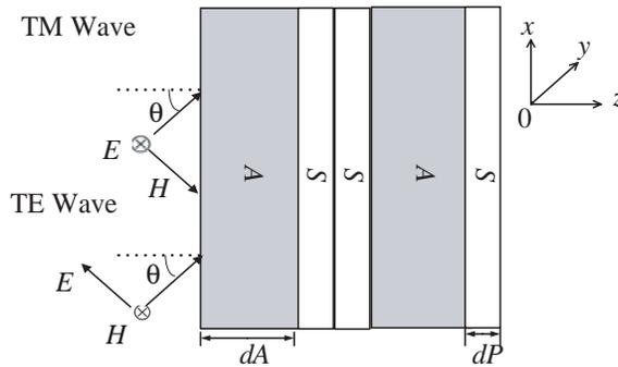
**Figure 1.** Schematic diagram of 4th order Fibonacci quasi-periodic 1D SDPCs consisting of dielectric ( $A$ ) and superconductor ( $S$ ) under any incidence angle ( $\theta$ ) for TE and TM waves.
