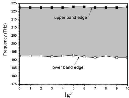
**Figure 13.** The frequency range of OBGs for Fibonacci quasi-periodic 1D SDPCs as a function of  $\lg\gamma$  at  $T = 6\text{ K}$ . The gray area is OBG.
