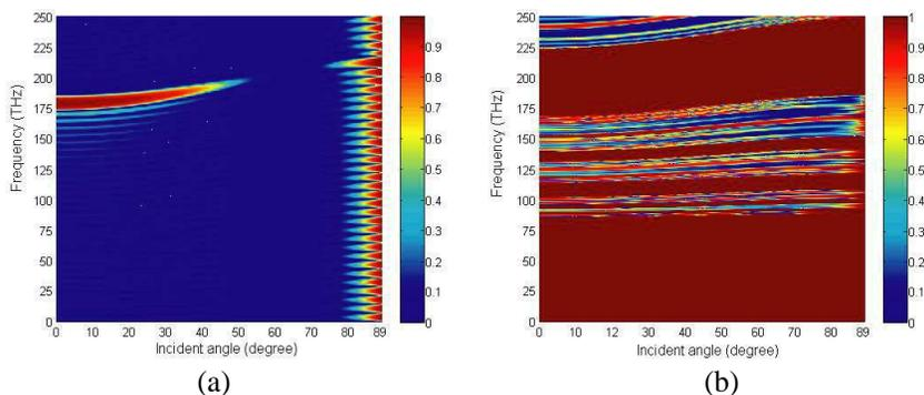
**Figure 2.** Photonic band structure of (a) 1D binary dielectric PCs, and (b) 1D Fibonacci quasi-periodic SDPCS in terms of angular frequency and incidence angle for TM polarization. The background corresponds to Bragg gaps or high-reflectance ranges.
