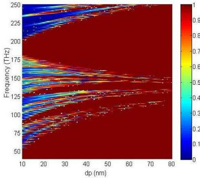
**Figure 6.** Reflection coefficients of Fibonacci quasi-periodic 1D SDPCs versus frequency as a function of the superconductor thickness at normal incidence.
