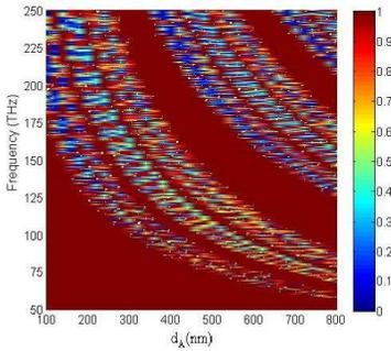
**Figure 8.** Reflection coefficients of Fibonacci quasi-periodic 1D SDPCs versus frequency as a function of the thickness of dielectric layer at normal incidence.
