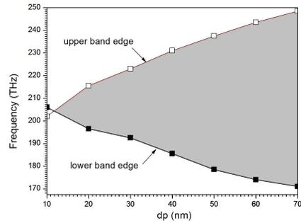
**Figure 7.** The frequency range of the OBG for Fibonacci quasi-periodic 1D SDPCs as a function of the superconductor thickness. The gray area is OBG.
