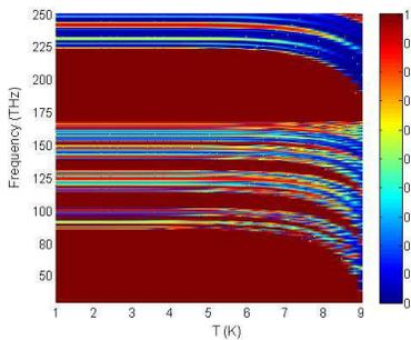
**Figure 10.** Reflection coefficients of Fibonacci quasi-periodic 1D SDPCs versus frequency as a function of the ambient temperature.
