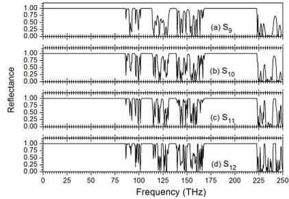
**Figure 5.** Normal incident reflection spectra for the different Fibonacci orders as a function of the frequency with (a)  $S_9$ , (b)  $S_{10}$ , (c)  $S_{11}$ , and (d)  $S_{12}$ .
