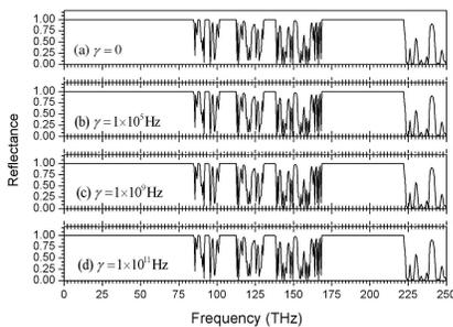
**Figure 12.** Reflectance of Fibonacci quasi-periodic 1D SDPCs versus frequency at normal incidence with different damp coefficient of superconductor layers at  $T = 6\text{ K}$ .
