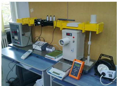
Figure 6. Laboratory installation used for microwave/cold/hot air processing of granular dielectric materials.
