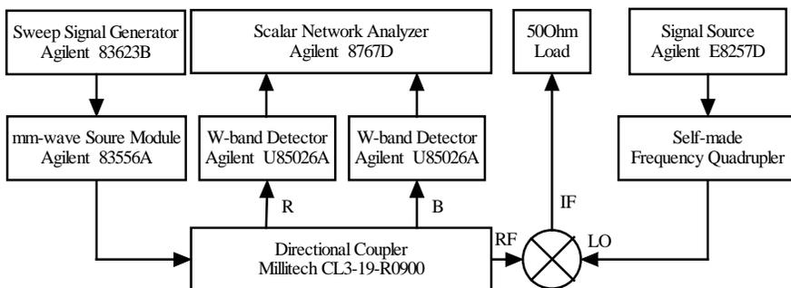
Figure 11. Block diagram for RF return loss measurement.
