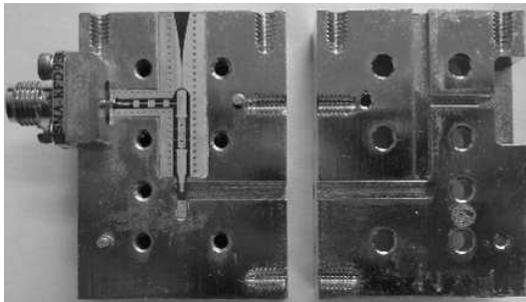
**Figure 9.** Photograph of the U-band finline mixer.
