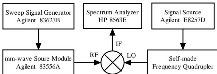
Figure 10. Block diagram for conversion loss measurement.
