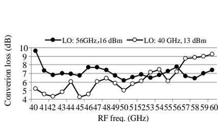
Figure 12. Measured conversion loss.
