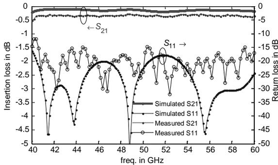
**Figure 7.** Simulated and measured  $S$ -parameters of the IF block in 40  $\sim$  60 GHz range.
