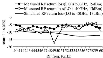
Figure 13. Measured return loss of RF port.
