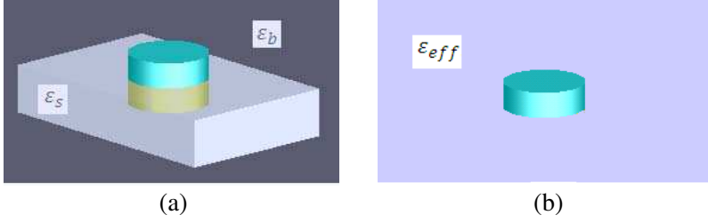
Figure 2. (a) The NP in a medium with electric permittivity of \varepsilon_b (green disk on top of the substrate) and its mirror image inside the substrate with electric permittivity of \varepsilon_s (dark yellow disk inside the substrate). (b) Representation of the combined substrate/medium shown in (a) by an infinite medium with effective permittivity of \varepsilon_{eff} in which only the NP is embedded.
