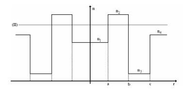
Figure 1. Index of refraction profile for RII structure.
