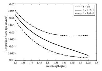
Figure 4. Dispersion slope vs. wavelength at  $\lambda_0 = 1.55 \,\mu\text{m}$ .
