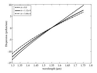
Figure 3. Dispersion vs. wavelength at  $\lambda_0 = 1.55 \,\mu\text{m}$ .
