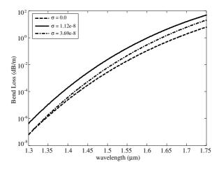
Figure 6. Bending loss (dB/m) Vs wavelength ( $\mu$ m) with 1 cm radius of the curvature.
