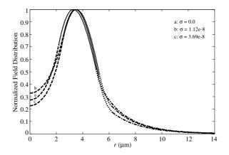
Figure 5. Normalized field distribution versus the radius of the fiber at  $\lambda = 1.55 \,\mu\text{m}$  with  $\sigma$  as parameter (dashed, solid line, dotted, and dashed-dotted curve represent the core and three cladding layers, respectively).
