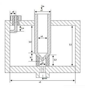
Figure 2. Configuration of the proposed coaxial cavity resonator.
