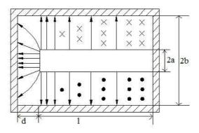
**Figure 1.** Electromagnetic field distribution of capacitive loaded coaxial cavity.
