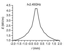
Figure 6. Electric field distribution on the axis of the resonator in the area of liquid.
