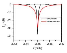
Figure 9. Measured and simulated return loss of the proposed resonator.
