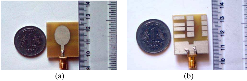
Figure 12. Fabricated prototype antenna. (a) Front view, (b) back view.
