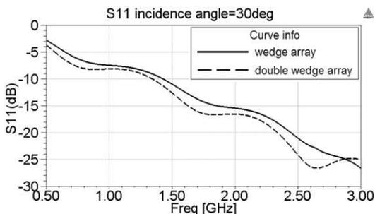
**Figure 5.** Comparison of wedge and double wedge array reflection coefficients for the 30 degrees angle of incidence at frequency range of 0.5–3 GHz.
