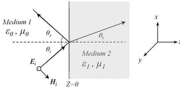
**Figure 1.** Plane wave incidence on lossy dielectric.
