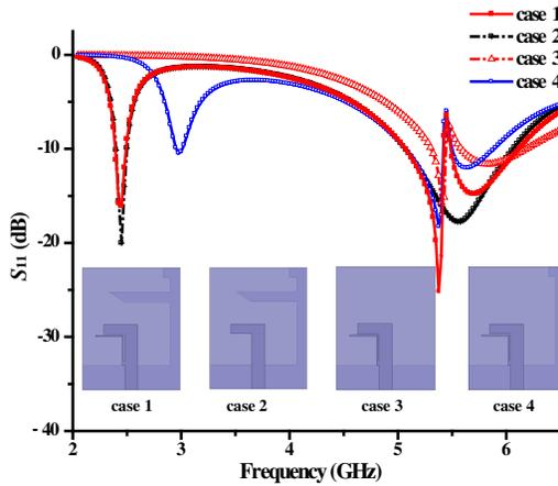
**Figure 5.**  $S_{11}$  curves of the proposed antenna in the different cases.
