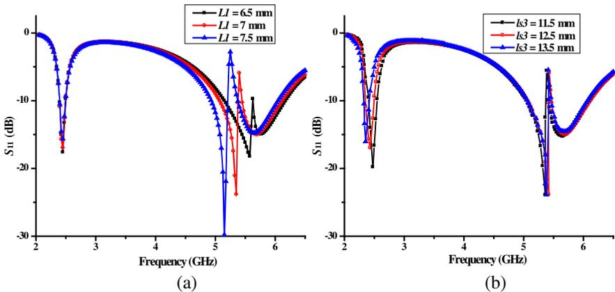
**Figure 6.** Simulated  $S_{11}$  variations for the proposed antenna of different lengths  $L1$  and  $ls3$ . (a)  $L1$ . (b)  $ls3$ . (Other parameters are the same as in Table 1).
