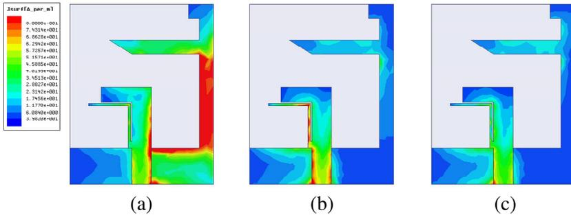
**Figure 4.** Simulated surface current distributions at different frequencies. (a) 2.425 GHz. (b) 5.35 GHz. (c) 5.75 GHz.
