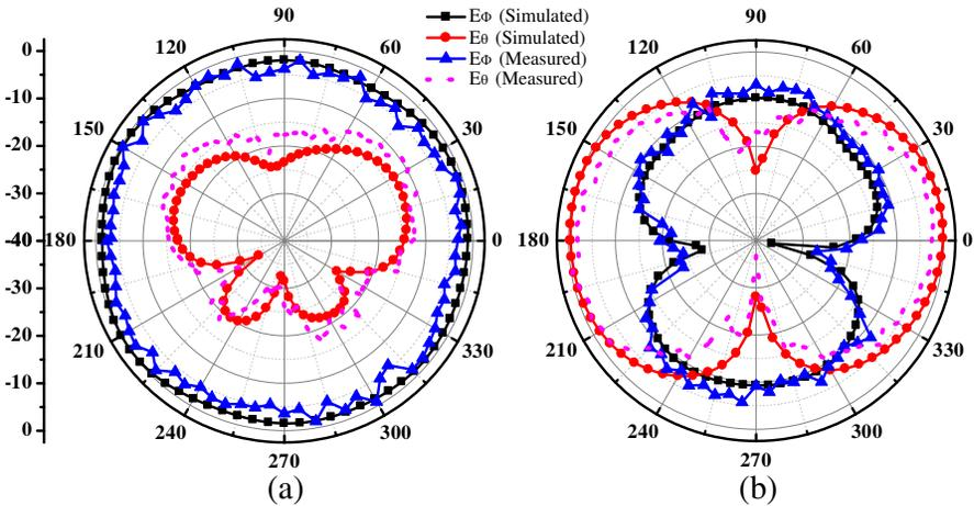
**Figure 9.** Measured and simulated normalized radiation patterns for the proposed antenna at 5.75 GHz. (a)  $x$ - $z$  plane. (b)  $y$ - $z$  plane.
