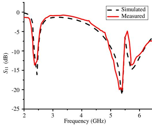
**Figure 3.** Simulated and measured  $S_{11}$  curves of the triple-band monopole antenna.
