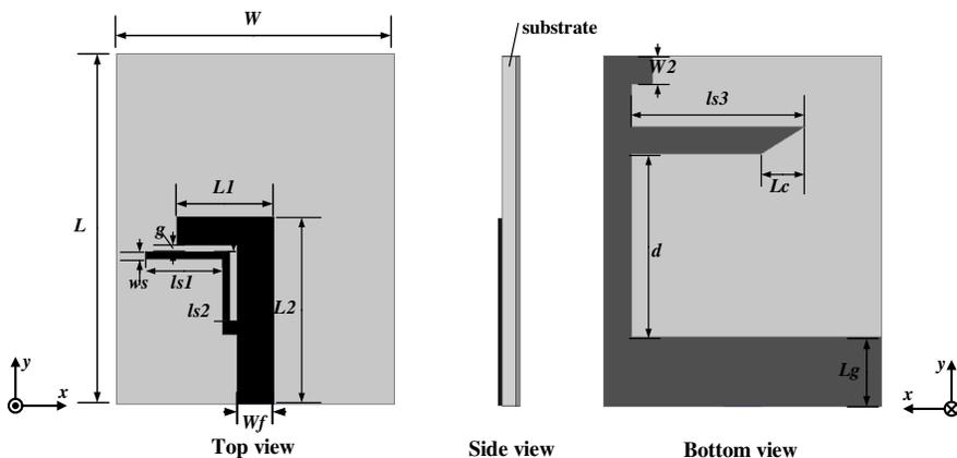
**Figure 1.** Geometry and dimensions of the proposed antenna.
