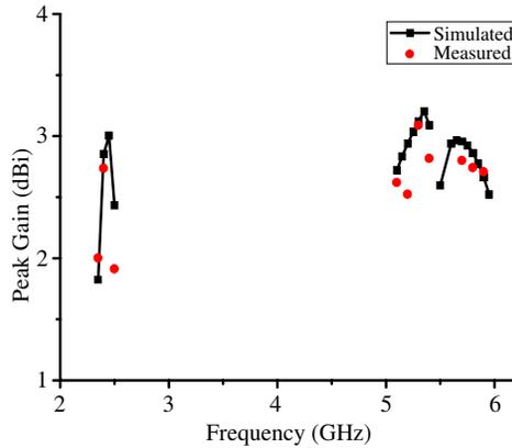
**Figure 10.** Measured and simulated peak antenna gains of the proposed antenna for the triple bands.
