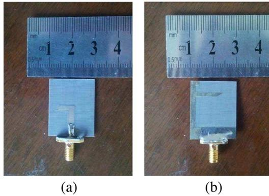
**Figure 2.** Photograph of the fabricated printed triple-band monopole antenna with optimal dimensions. (a) Top view. (b) Bottom view.
