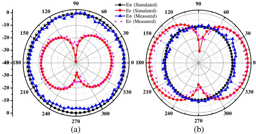
**Figure 7.** Measured and simulated normalized radiation patterns for the proposed antenna at 2.425 GHz. (a)  $x$ - $z$  plane. (b)  $y$ - $z$  plane.
