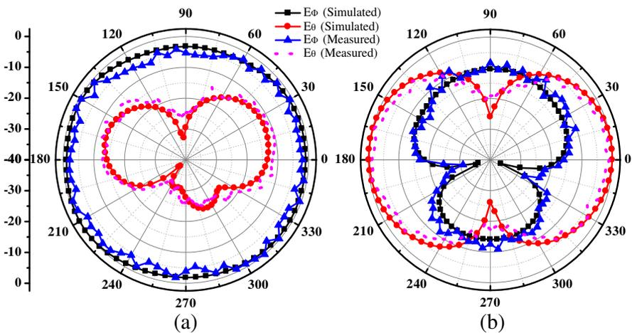
**Figure 8.** Measured and simulated normalized radiation patterns for the proposed antennas at 5.35 GHz. (a)  $x$ - $z$  plane. (b)  $y$ - $z$  plane.
