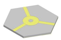
Figure 5. The simulated geometry of design 1 with three ports emanating from the outer radius an equal distance apart ( $\theta_2 = \theta_3 = 2\pi/3$ ).
