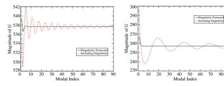
Figure 3. Comparison of convergence of  $G(a_s, \phi_i; a_s, \phi')$  as calculated by Equations (18) and (32) for  $\phi_i - \phi' = 1.0$  rad.
