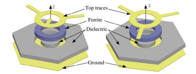
Figure 1. Geometrical and material structure of candidate ring circulators. Note that z = 0 is located coincident with the ground plane.
