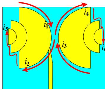
**Figure 5.** Edge currents on the antenna radiators.
