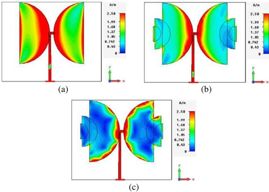
**Figure 4.** Simulation results of the metal surface current. (a)  $f = 3.0$  GHz, (b)  $f = 2.5$  GHz, (c)  $f = 16$  GHz.
