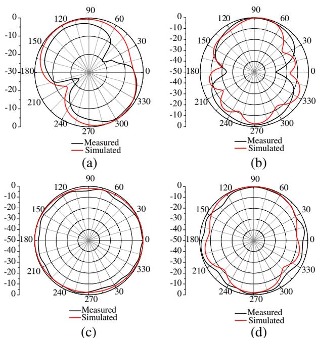
**Figure 10.** Tested results of the antenna. (a) Tested result of the antenna radiation pattern in  $E$ -plane (2.5 GHz). (b) Tested result of the antenna radiation pattern in  $E$ -plane (16 GHz). (c) Tested result of the antenna radiation pattern in  $H$ -plane (2.5 GHz). (d) Tested result of the antenna radiation pattern in  $H$ -plane (16 GHz).
