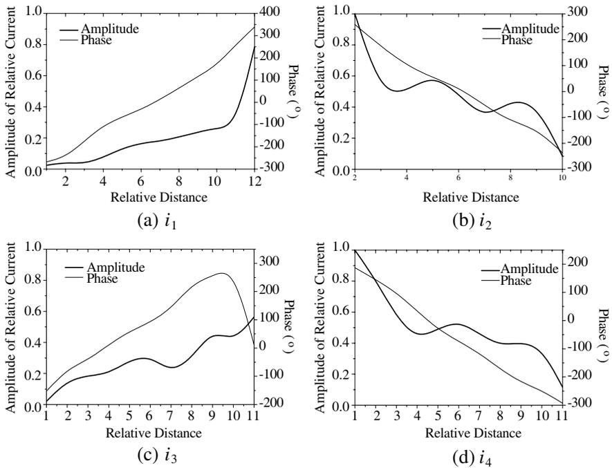
**Figure 7.** The amplitude and phase of the edge currents on radiators (16 GHz).
