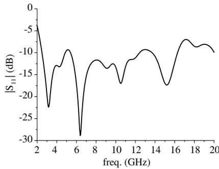
**Figure 2.** The simulation result of  $S$ -parameter.
