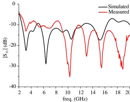
**Figure 9.** Tested  $|S_{11}|$  of the antenna prototype.
