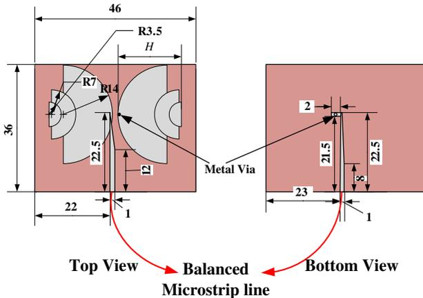
**Figure 1.** Printed antenna with semicircular combinatorial symmetrical radiators ( $H = 18.1 \text{ mm}$ ).
