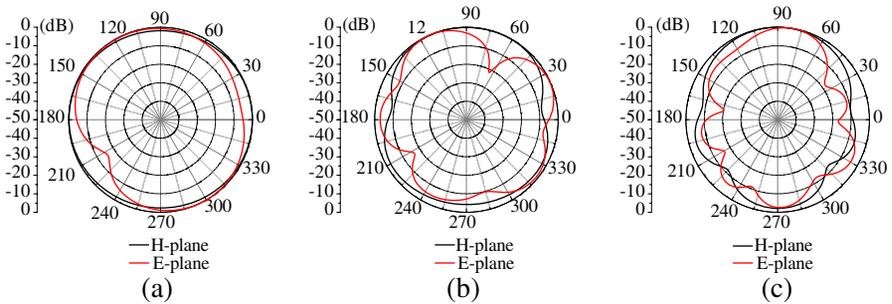
**Figure 3.** Radiation patterns of the printed antenna with combinatorial semicircular symmetrical dipoles. (a) 2.5 GHz, (b) 7 GHz, (c) 16 GHz.
