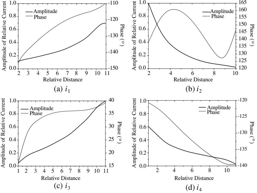
**Figure 6.** The amplitude and phase of edge currents on the radiators (2.5 GHz).
