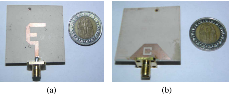
Figure 2. Photograph of fabricated E-shaped antenna. (a) Top view. (b) Bottom view.
