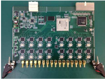
Figure 4. The data acquisition unit in BHU-2D.
