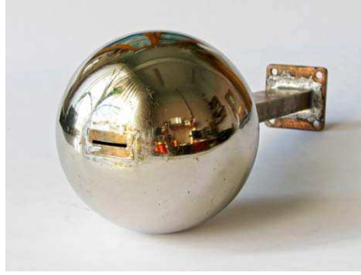
Figure 3. The prototype model of the spherical antenna.
