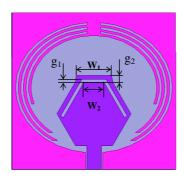
Figure 7. The configurations of the multiband antenna with two notch bands.
