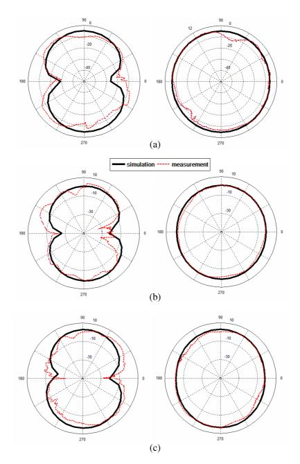
**Figure 12.** Measured and simulated *E*-plane and *H*-plane radiation patterns at (a) 2.45 GHz, (b) 4.5 GHz and (c) 7 GHz.
