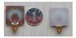
Figure 9. Photo of the proposed antenna: Top view and bottom view.
