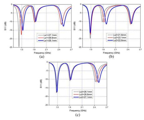
Figure 4. The simulated reflection coefficients of the multi-band antenna with (a)  $L_{s2} = 22.1 \text{ mm}$  and  $L_{s3} = 16.1 \text{ mm}$  for various  $L_{s1}$ , (b)  $L_{s1} = 26.6 \text{ mm}$  and  $L_{s3} = 16.1 \text{ mm}$  for various  $L_{s2}$ , (c)  $L_{s1} = 26.6 \text{ mm}$  and  $L_{s2} = 22.1 \text{ mm}$  for various  $L_{s1}$ .
