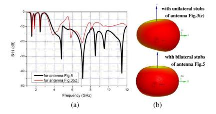
Figure 6. Comparison of unilateral and bilateral stubs: (a) The reflection coefficients, (b) the simulated radiation far field patterns at 2.45 GHz.
