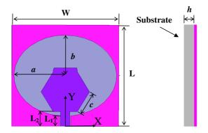
Figure 1. The front view of the primitive antenna, the side view of the primitive antenna.
