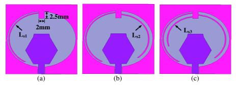
**Figure 3.** (a) The UWB antenna with adding stub  $L_{s1}$ . (b) The UWB antenna with adding stub  $L_{s1}$  and  $L_{s2}$ . (c) The UWB antenna with adding stub  $L_{s1}$ ,  $L_{s2}$  and  $L_{s3}$ .
