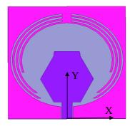
Figure 5. The structure of multiband antenna.
