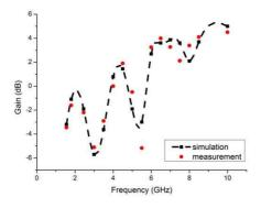
Figure 11. The measured and simulated gains of the proposed antenna.
