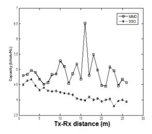
Figure 10. Comparison of the capacity for MIMO and SISO in LOS condition.
