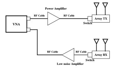
Figure 2. Measurement setup.
