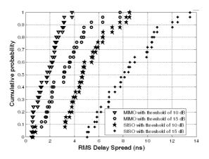
Figure 7. Cumulative distribution function for two thresholds for MIMO and SISO in LOS.
