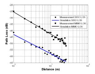
Figure 4. Path loss versus distance in LOS scenario.
