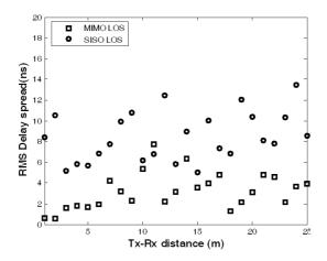
Figure 8. Comparison of the delay spread for MIMO and SISO for a threshold of 15 dB in LOS.
