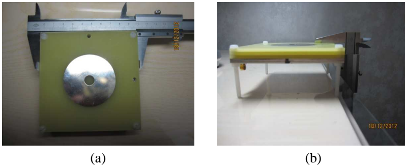
Figure 5. Photo of the designed antenna. (a) Front view. (b) Side view.
