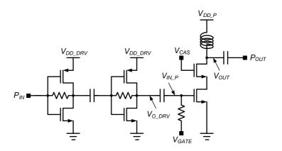
Figure 2. Simplified schematic of a general power amplifier.
