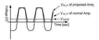
Figure 6. Comparison of the input voltage waveforms of the power stages.
