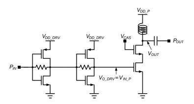
Figure 4. Simplified schematic of a power amplifier without an interstage capacitor.
