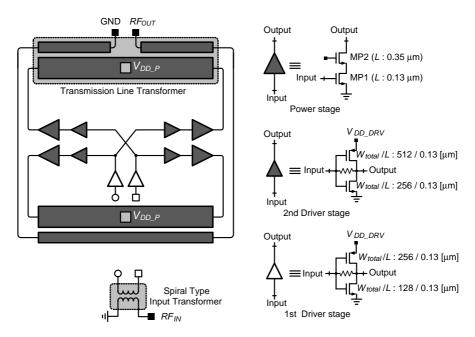
Figure 9. Schematic of the designed power amplifier.
