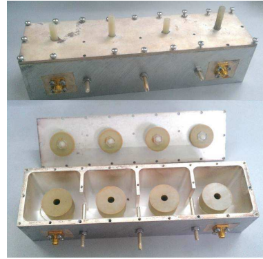
Figure 15. Photographs of manufactured four-pole DR filter.
