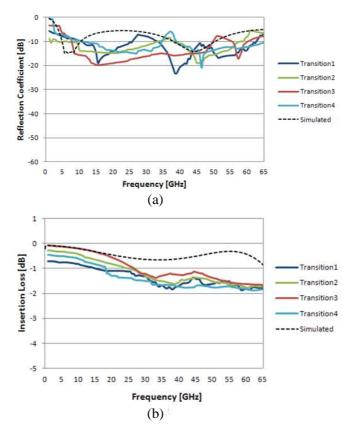
**Figure 8.** Measured results of micro-coaxial transition vs. simulated response with substrate integration. (a) Reflection coefficient and (b) insertion loss.
