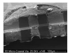
Figure 4. Cross-section SEM image of micro-coaxial transition post through-hole metallization.
