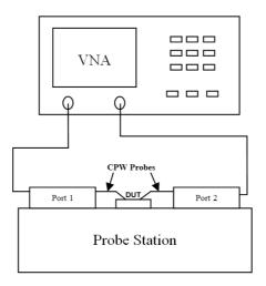
Figure 6. Illustration of test setup used for RF characterization of micro-coaxial transition.
