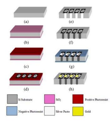
Figure 2. Fabrication process sequence for the vertical microcoaxial transition. (a) Si substrate, (b) SiO<sub>2</sub> grown on the substrate, (c) photoresist deposited for patterning, (d) pattern transfer by photolithography, (e) removal of SiO<sub>2</sub> layer for etching and coaxial vias formed using deep reactive ion etching, (f) metallization of holes, (g) pattern transfer for CPW lines, and (i) CPW line metal deposition. steps involved in the fabrication process.
