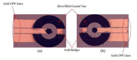
**Figure 5.** Microscopic images of fabricated micro-coaxial transition with gold deposited CPW lines. (a) Front side and (b) backside.
