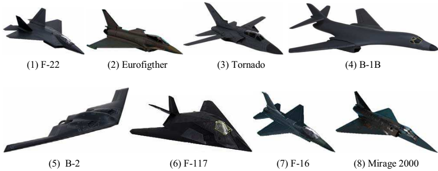
Figure 4. Scale-reduced aircraft models used into anechoic chamber experiment.
