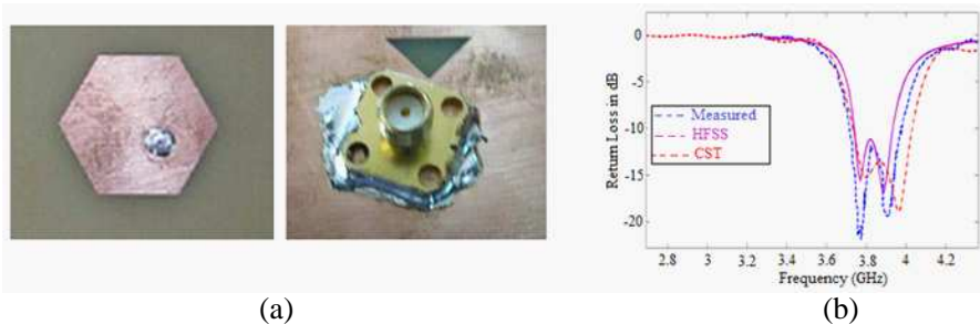
Figure 5. (a) Photograph of HMP with slot in ground. (b) Measured and simulated return loss of HMP with slot in ground.
