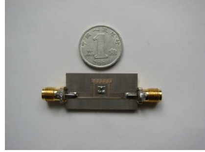
Figure 7. Photograph of the fabricated filter.
