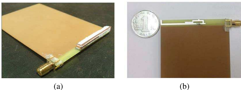
Figure 6. Prototype of the proposed multiband antenna (a) 3-D view, (b) strips on the board.
