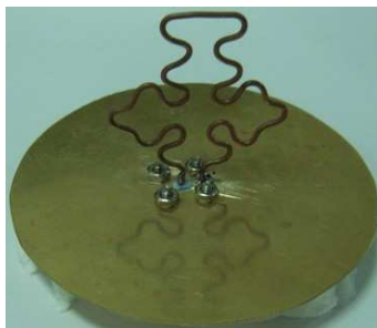
Figure 17. Prototype of \mathbf{K}_2 CAKC folded monopole (SMA with 4-holed square flange).
