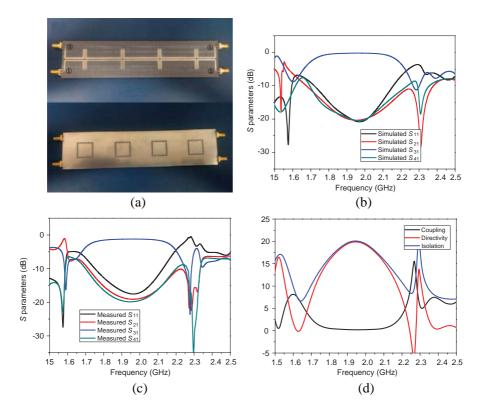
**Figure 7.** (a) Top (upper) and bottom (lower) sides of the fabricated coupler with parameters: R = 20 mm, w = 1 mm, g = 0.5 mm,  $w_1 = 0.3 \text{ mm}$ ,  $L_1 = 1.8 \text{ mm}$ , d = 0.2 mm, L = 18 mm, N = 21, the spacing between the two CRLH TLs is s = 1 mm. (b) Full-wave simulated S parameters. (c) Measured S parameters, and (d) the three quantities characterizing the coupler.
