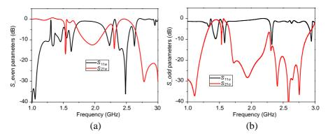
**Figure 5.** EM simulated S-parameters for the even and odd modes of the coupler shown in Figure 7. (a) Even mode. (b) Odd mode.
