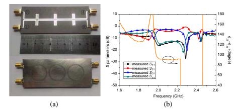
**Figure 8.** (a) Prototype of the 3-dB backward directional coupler constituted of two CRLH TLs with parameters:  $R = 12 \text{ mm}, w = 0.3 \text{ mm}, g = 0.3 \text{ mm}, w_1 = 0.2 \text{ mm}, L_1 = 1.8 \text{ mm}, d = 0.2 \text{ mm}, L = 11 \text{ mm}, N = 17$ , the spacing between the two CRLH lines is s = 0.5 mm. (b) Measured results.
