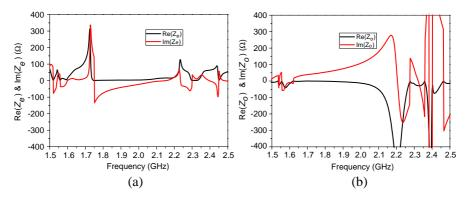
**Figure 6.** EM simulated even/odd characteristic impedances (real/imaginary parts) for the coupler shown in Figure 7. (a) Even mode. (b) Odd mode.
