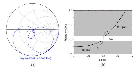
**Figure 2.** (a) Representation of the simulated reflection coefficient for the structures shown in Figure 1 on Smith Chart. (b) Simulated dispersion diagram obtained by Equation (8) with phase unwrapping.
