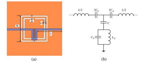
**Figure 1.** Topology of the unit cell of (a) CSRR-based CRLH transmission line and (b) equivalent circuit model.
