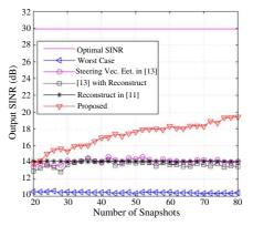
Figure 3. Output SINR versus SNR of the second example, T = 30.
