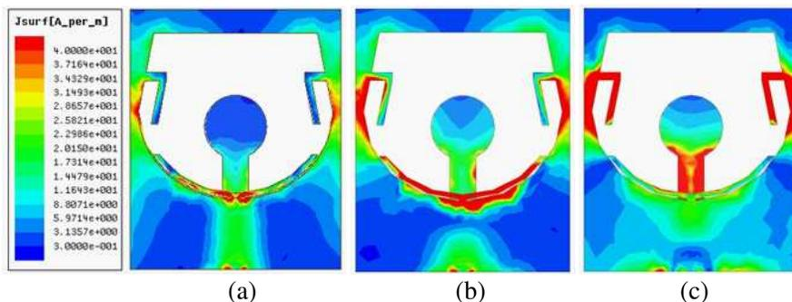
**Figure 3.** Simulated surface current distributions of the proposed antenna at (a) 2.5, (b) 3.5, and (c) 5.5 GHz.
