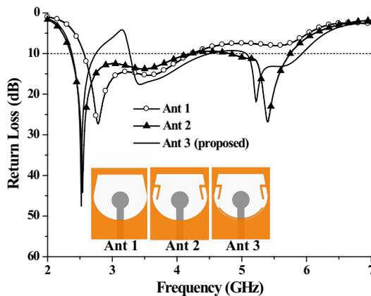
**Figure 2.** Geometry and simulated return loss of various antennas.
