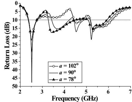
**Figure 7.** Simulated return loss with varying the angle of inverted-L strip  $a$ .
