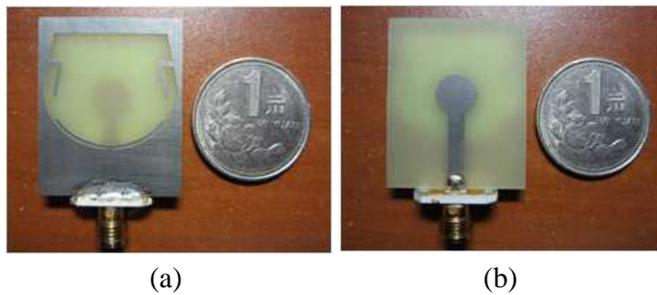
**Figure 8.** Photograph of the fabricated antenna. (a) Front view, (b) back view.
