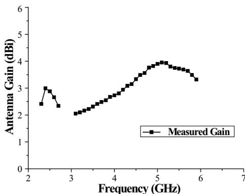
**Figure 11.** Measured antenna gain for the proposed antenna.
