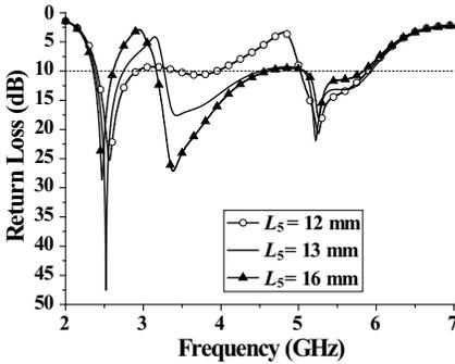
**Figure 4.** Simulated return loss with varying the elliptical-arc-shaped stub's length  $L_5$ .
