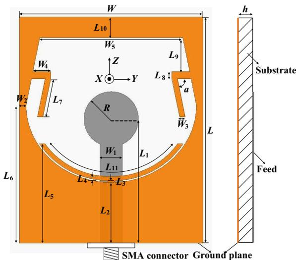
**Figure 1.** Geometry of proposed microstrip slot antenna.
