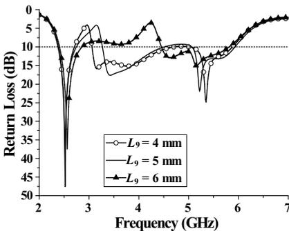
**Figure 6.** Simulated return loss with varying the position of inverted-L strip  $L_9$ .
