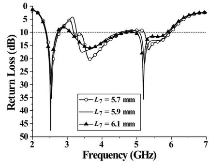
**Figure 5.** Simulated return loss with varying the inverted-L strip's length  $L_7$ .
