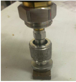
Figure 5. Dielectric probe was used to measure the dielectric properties of the RHCNT microwave absorber.
