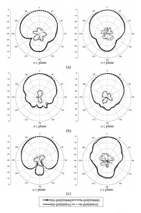
**Figure 8.** Measured and simulated radiation patterns at (a) 2.2 GHz, (b) 2.7 GHz, and (c) 3.1 GHz.
