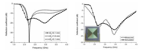
Figure 5. Effect of the CPW structure on the antenna performance.
