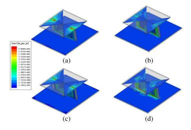
Figure 2. Current distributions of the proposed antenna at different times. (a) t = 0; (b) t = T/4; (c) t = T/2; (d) t = 3T/4.
