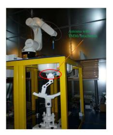
**Figure 7.** Photograph of the real measurement system for the antenna with the TMMs in the tilted position.
