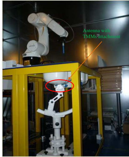
Figure 7. Photograph of the real measurement system for the antenna with the TMMs in the tilted position.
