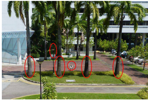
Figure 10. Ground truth of the target area with main targets: four palm trees, one street lamp post, and one trihedral corner reflector (circled in red).
