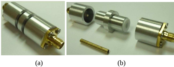
Figure 12. Ad-hoc connector prototype. (a) Plugged. (b) Unplugged.
