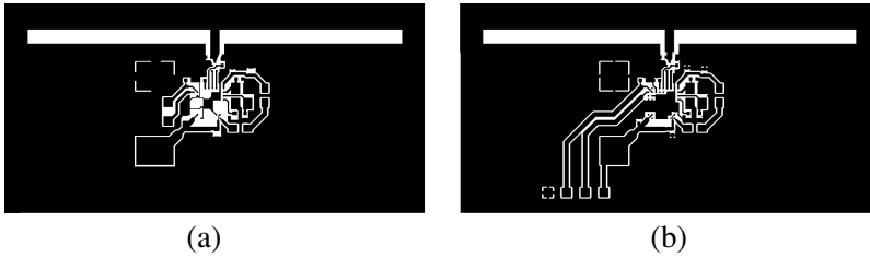
Figure 8. Sensor layouts for antenna measurements. The size of the sensors is 45\text{ mm} \times 22.5\text{ mm} . (a) Sensor 1, (b) sensor 2.
