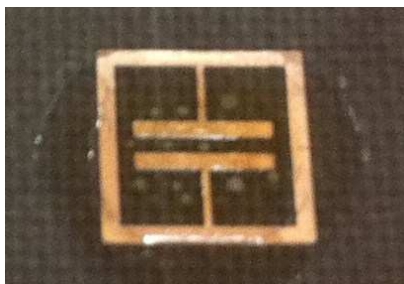
Figure 14. Photo of fabricated ELC resonator with PVA coating.
