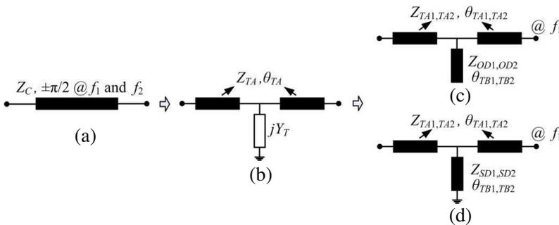
**Figure 7.** The desired dual-band branch-line and its implementing T-network circuit structure.
