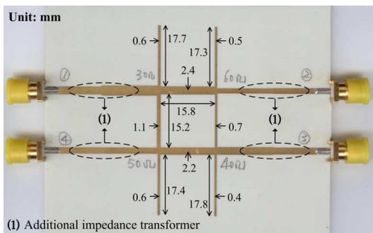
**Figure 15.** Photograph and dimensions of the fabricated coupler based on open-circuited pi-network.
