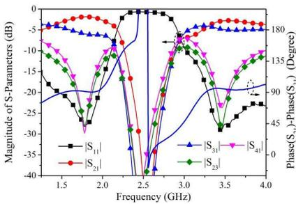
**Figure 17.** The measured  $S$ -parameters and phase difference of the coupler prototype based on open-circuited pi-network.
