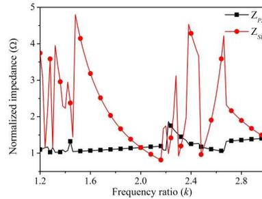
**Figure 6.** Normalized impedances of the short-circuited pi-network versus frequency ratio.
