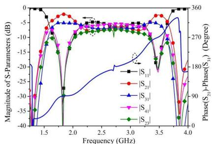
**Figure 14.** The EM simulated *S*-parameters and phase difference of the coupler prototype based on open-circuited T-network.
