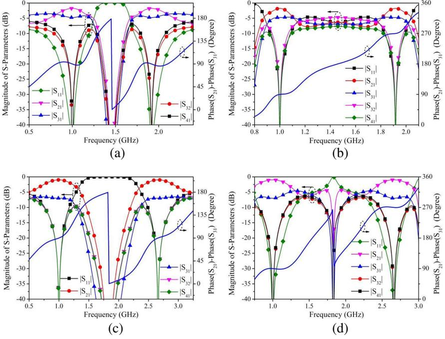
**Figure 12.** The calculated  $S$ -parameters and phase difference of the couplers, (a) Coupler A, (b) Coupler B, (c) Coupler C, (d) Coupler D.
