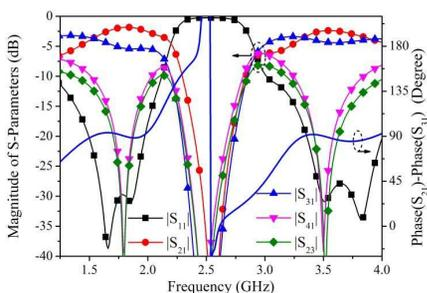
**Figure 13.** The EM simulated *S*-parameters and phase difference of the coupler prototype based on open-circuited pi-network.
