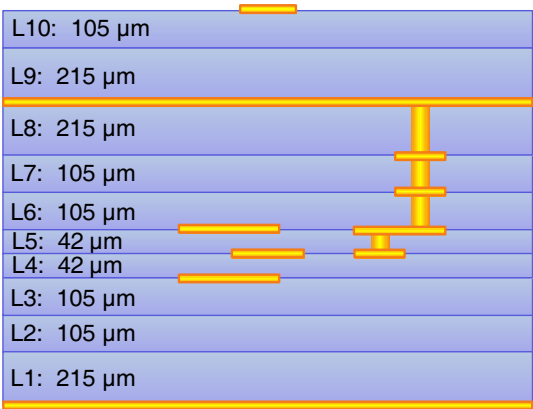
Figure 3. LTCC layer structure, DuPont-943 substrate.
