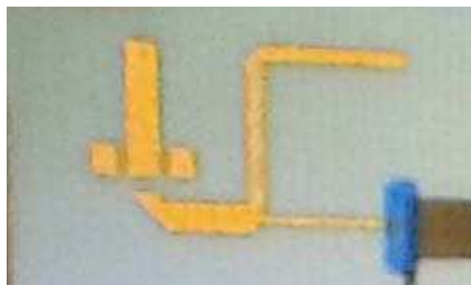
Figure 14. Detail of one output port with ground patches for probe positioning.
