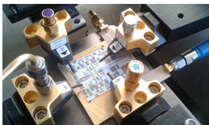
Figure 13. Test-bench for the measurement of the scattering parameters.
