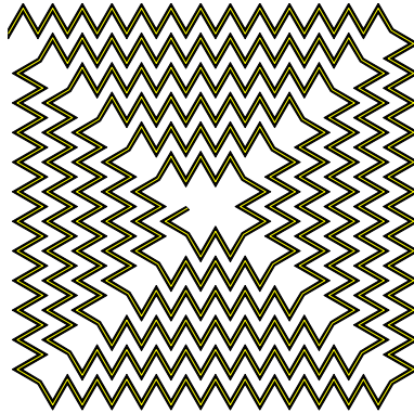
Figure 4. Planar zig-zag spiral inductor of square shape (side dimension l_0 ) with its axis.
