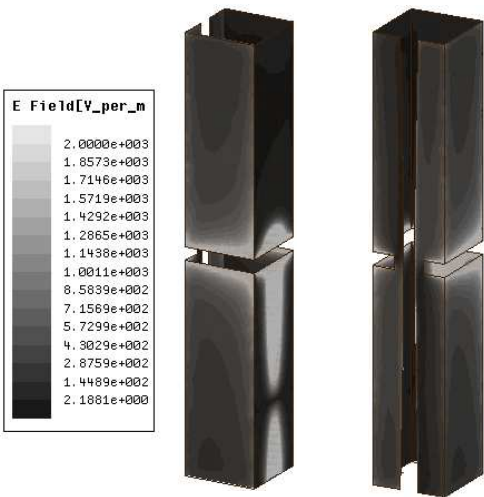
Figure 2. Electric field magnitude distribution of the VP mode fed by port 1 at 2.44 GHz.
