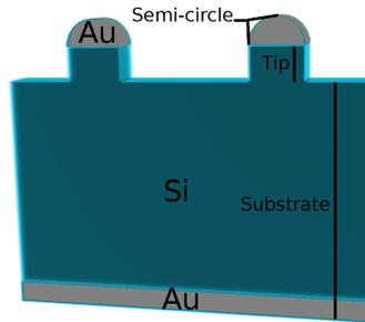
**Figure 3.** Sample photonic structure periodic in one dimension. Structure parameters: period — 860 nm, silicon bulk layer thickness — 1000 nm, silicon tips high — 160 nm, golden underlayer thickness — 100 nm, golden semi-circles radius — 130 nm.
