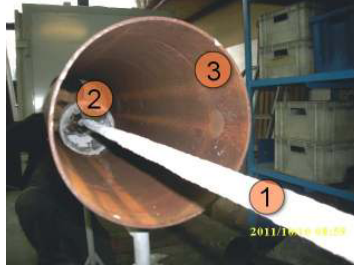
Figure 1. Induction heater setup: 1 — high current busduct (bandaged), 2 — inner inductor, 3 — workpiece (heated cylindrical element).
