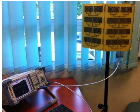
Figure 9. Measurement of antenna reflection coefficient in hexagon structure.
