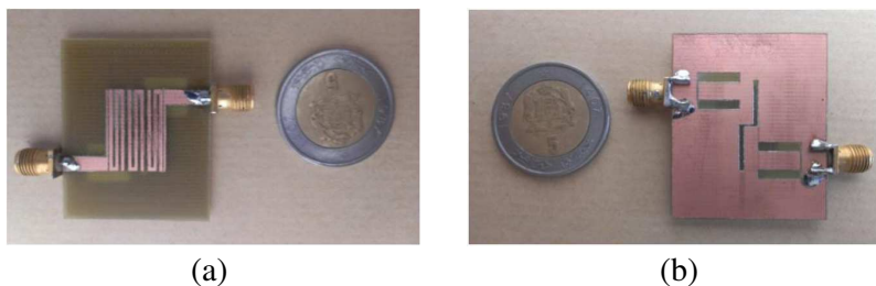
Figure 17. Fabricated three-pole N lines BPF with three-cell DGS. (a) Top view. (b) Bottom view.
