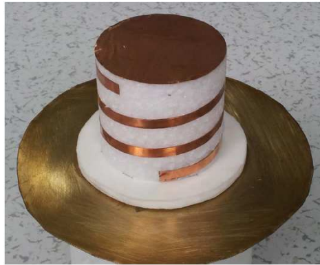
Figure 2. The fabricated antenna prototype.
