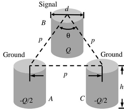
**Figure 2.** Three-wire transmission line with an angle  $\theta$  between the two ground conductor centers to the signal conductor center.
