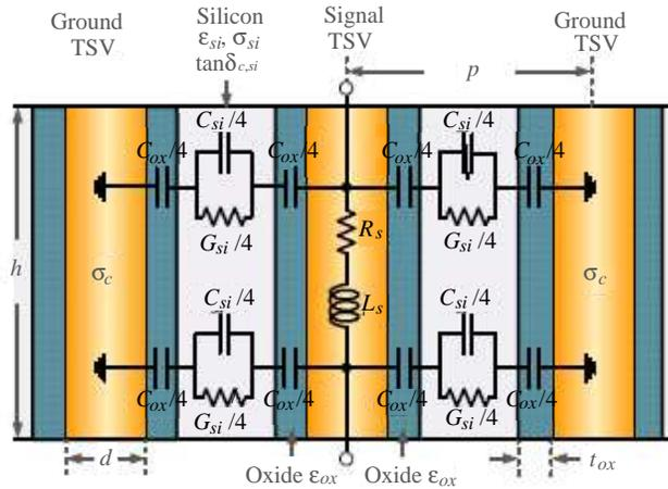
Figure 1. Physical modeling of a SE TSV in GSG configuration.
