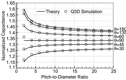
**Figure 3.** Comparison of the normalized capacitance of three-wire transmission.
