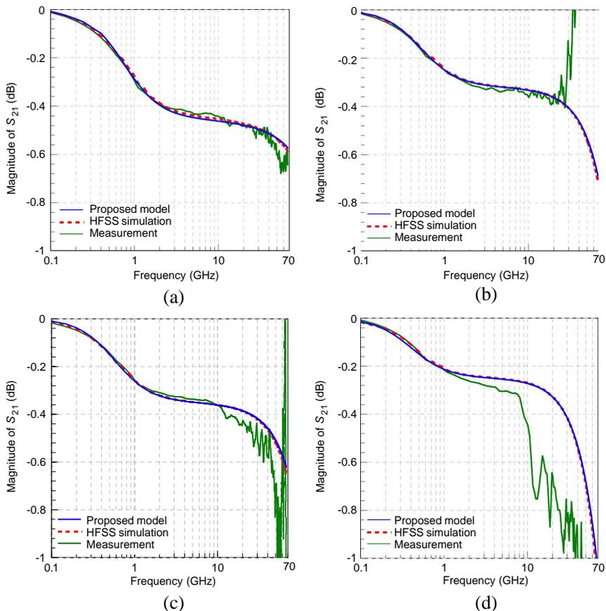
**Figure 9.** Comparison of the Magnitude of  $S_{21}$  among proposed model, HFSS simulation and measurement. (a)  $p/d = 5$ , GSG. (b)  $p/d = 5$ , GS. (c)  $p/d = 10$ , GSG. (d)  $p/d = 10$ , GS.
