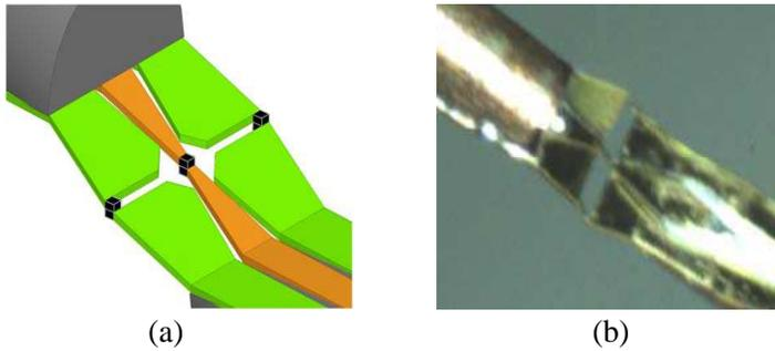
**Figure 7.** Illustration of the direct contact between the upper and lower probes as a thru kit. (a) 3-D geometry. (b) Photograph.
