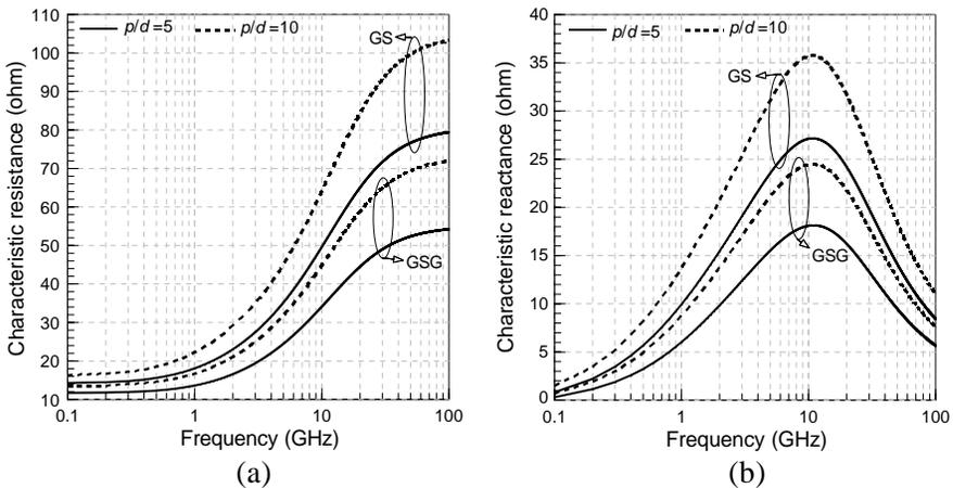
**Figure 5.** Complex characteristic impedance of SE TSVs in the GS and GSG configurations with  $\theta = 180^\circ$ . (a) Characteristic resistance  $R_0$ . (b) Characteristic reactance  $X_0$ .
