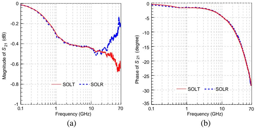
**Figure 8.** Comparison of the  $S_{21}$ -parameter measurement results between SOLT and SOLR calibration methods for the GSG configuration of TSV with  $p/d = 5$ . (a) Magnitude. (b) Phase.
