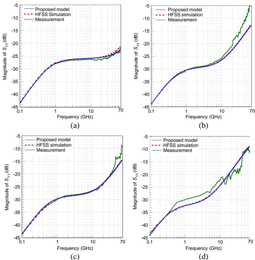
**Figure 10.** Comparison of the Magnitude of  $S_{11}$  among proposed model, HFSS simulation and measurement. (a)  $p/d = 5$ , GSG. (b)  $p/d = 5$ , GS. (c)  $p/d = 10$ , GSG. (d)  $p/d = 10$ , GS.
