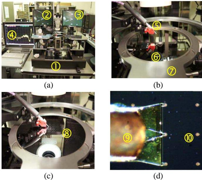
**Figure 6.** Double-sided probing system. (a) Front view of system. (b) Top and bottom probes used in the system. (c) TSV wafer probing. (d) Top view of TSV probing. (① Double-sided probe. station ② Top side display. ③ Bottom side display. ④ VNA display. ⑤ Top probe. ⑥ Bottom probe. ⑦ DUT holder. ⑧ Silicon interposer. ⑨ GSG-type probe. ⑩ TSV.).
