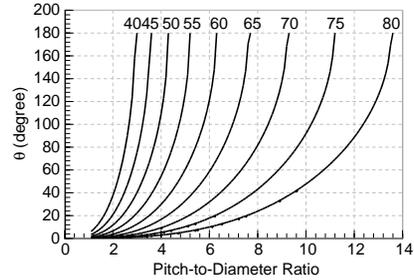
**Figure 4.** Root loci of constant characteristic impedances for a three-wire transmission line in an ideally lossless and homogeneous silicon medium.
